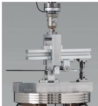
Fig. 3: Adjustable Mode I / Mode II proportions
