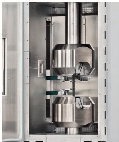
Fig. 2: makroXtens with long feeler sensors for tensile testing in a temperature chamber
