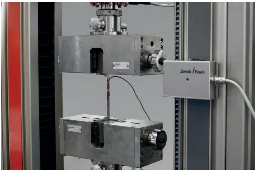
Fig. 4: Direct connection of the strain gauges to testControl II via a ready-configured control box.
