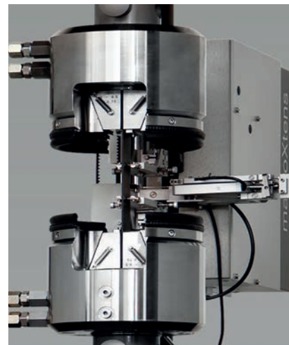
Fig. 4: makroXtens with transverse strain extensometer for tensile or in-plane shear (IPS) tests at RT
