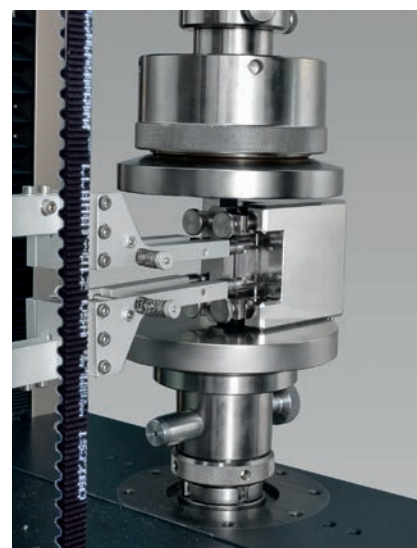
Fig. 5: makroXtens for module determination in an end loading compression test
