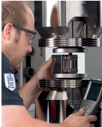
Fig. 2: End loading compression fixture to prEN 2850 and ASTM D695 (Boeing modified). The support block is centered to the compression axis using stops.
