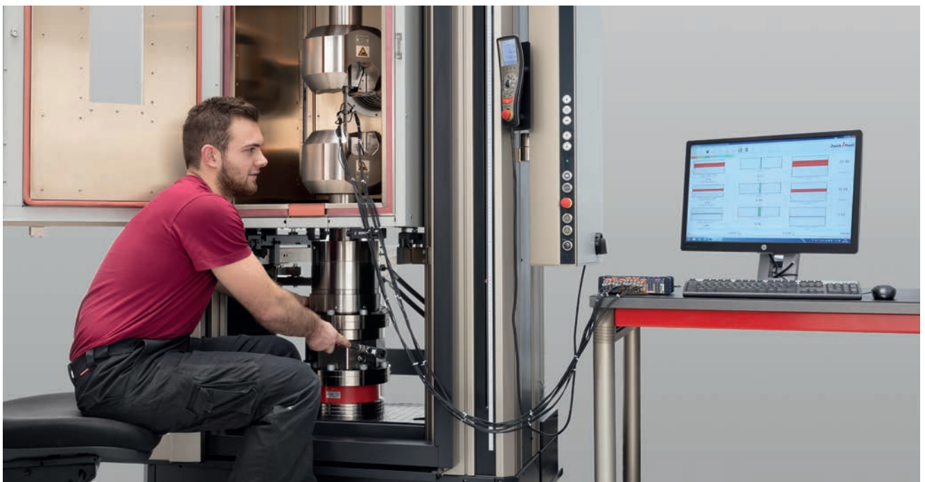
Fig. 1: Testing machine alignment and verification by a ZwickRoell technician using alignment in accordance with Nadcap AC 7122
