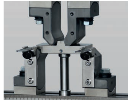
Fig. 5: Adjustment gauge for the 4-point flexure test arrangement
