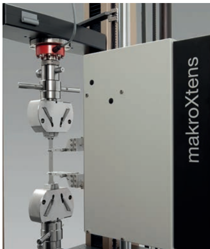
Fig. 1: Mechanical measurement, automatic attachment: makroXtens
