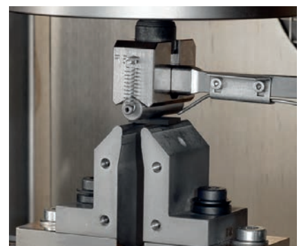
Fig. 5: Attachment of a temperature sensor close to the specimen
