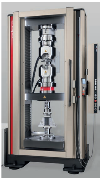
Fig. 2: During the compression test, the compressive residual strength of the specimen, and with that its damage tolerance, is determined. (Bottom: compression fixture to ASTM, DIN, Boeing; top: compression fixture to ISO, EN, Airbus.)
