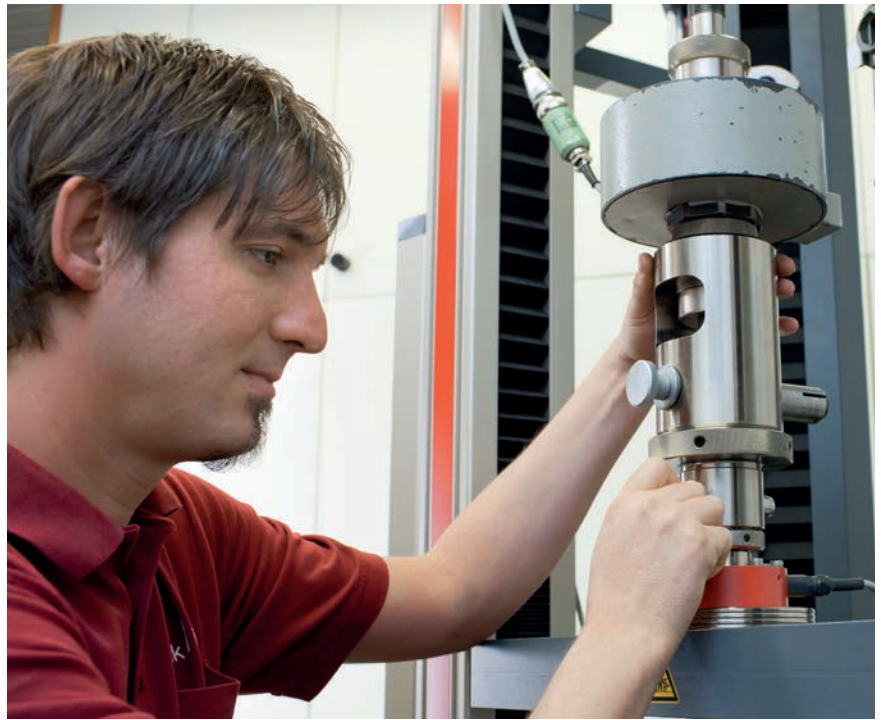
Fig. 2: Every load cell undergoes a ZwickRoell factory calibration as soon as it enters service on a testing machine.
