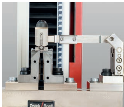
Fig. 3: Standard 10 mm adjustment gauge for exact alignment
