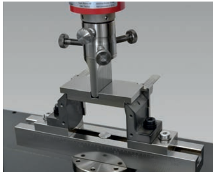
Fig. 3: Die and supports are clamped under load and aligned with the adjustment gauge.
