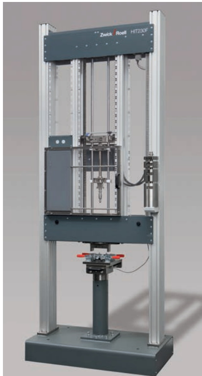
Fig. 1: HIT 230F drop weight tester with accessories for CAI pre-damaging
