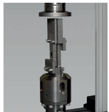
Fig. 5: OHC and FHC compression tests to ASTM require an anti-buckling support, which is used for shear loading with hydraulic specimen grips, and with end loading between compression platens.
