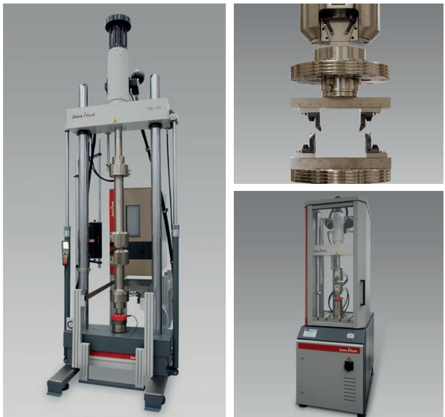
Fig. 2: Servohydraulic testing machine type HB100 (left) and HC compact (right). Modular design for dynamic and static testing of composite materials.
