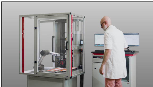
roboTest N for function testing on autoinjectors
