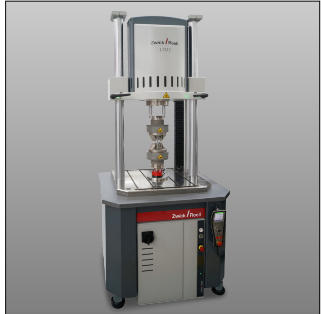
LTM 3 testing machine as floor-standing model with base
