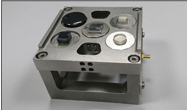
Steel specimen holder for 5 small specimen inserts, Ø 24 mm, insulated upper section
